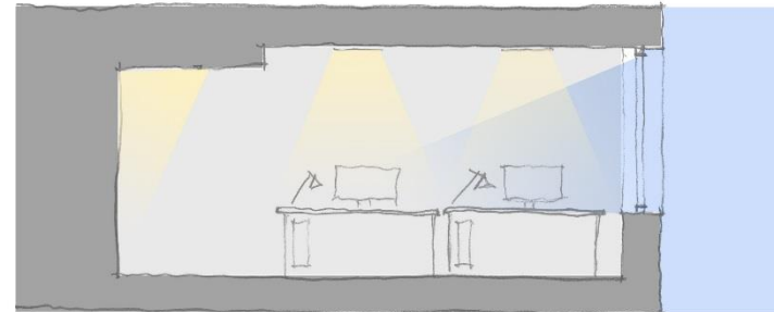
Standard daylight responsive dimming system at daytime
